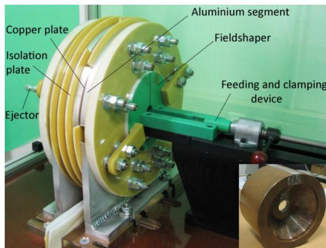
Figure 5 The coil without (left) and with (right) the field shaper in place
