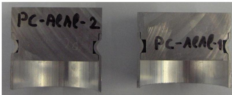
Figure 7 The effect of charging voltage on the deformation.
