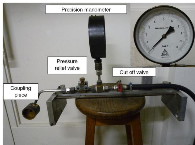
Figure 9 Air pressure test configuration [14]
