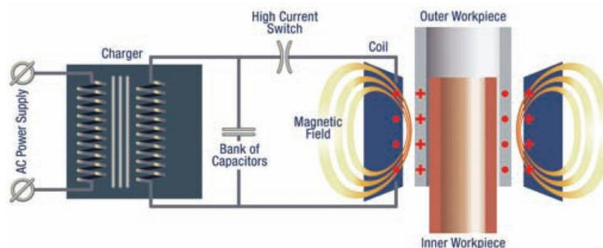
Figure 1 Principle of the electromagnetic pulse generator and the coil [2].
