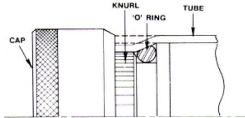
Figure 2 Suggestion for the use of an O-ring in EMP crimped joints [4]
