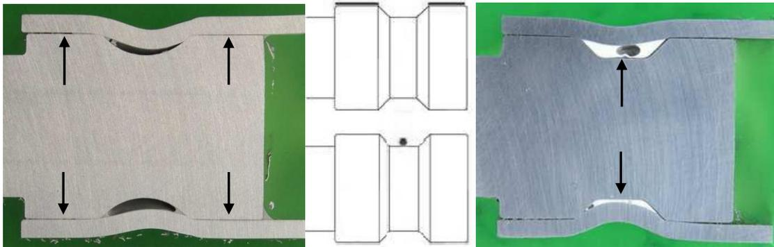
Figure 4 Cross sectioned EMP crimped joints sealed with adhesives [12].
