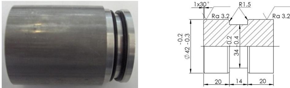
Figure 8 Mandrel with two O-rings in the corners of the groove (left) and drawing of a mandrel that will be used with adhesives (right)
